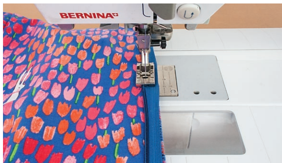
An invisible zipper foot uncurls the zipper chain as the machine stitches it in place.
