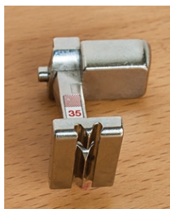
The bottom of an invisible zipper foot has two grooves and a small needle hole.
