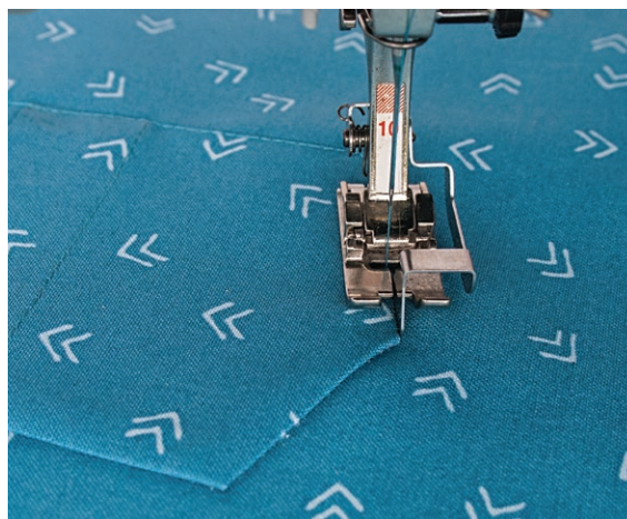
An edgestitching foot keeps topstitching evenly spaced from the edge of fabric.
