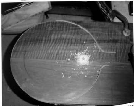
Tracing the bucket & tin onto the table leaf
