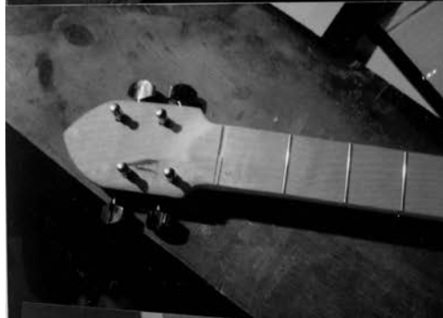
screwing on the tuning machines
