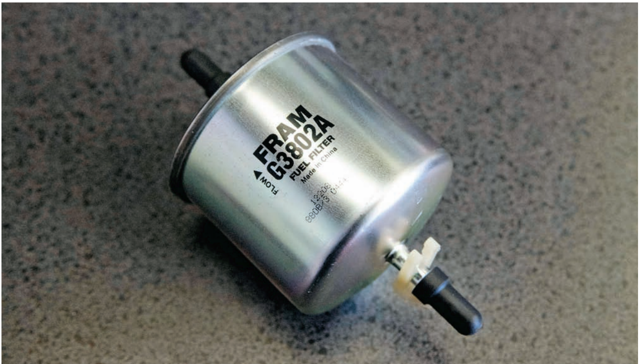
A typical automotive fuel filter: A small yet critical member of the fuel delivery system, the fuel filter has a massive responsibility for proper operation of the system. The fuel filter sifts out dirt and deposits that typically build up in fuel tanks. This operation is critical to proper operation of fuel injectors, small sprayers with orifices just a few thousandths of an inch in diameter that deliver fuel to the cylinders.
