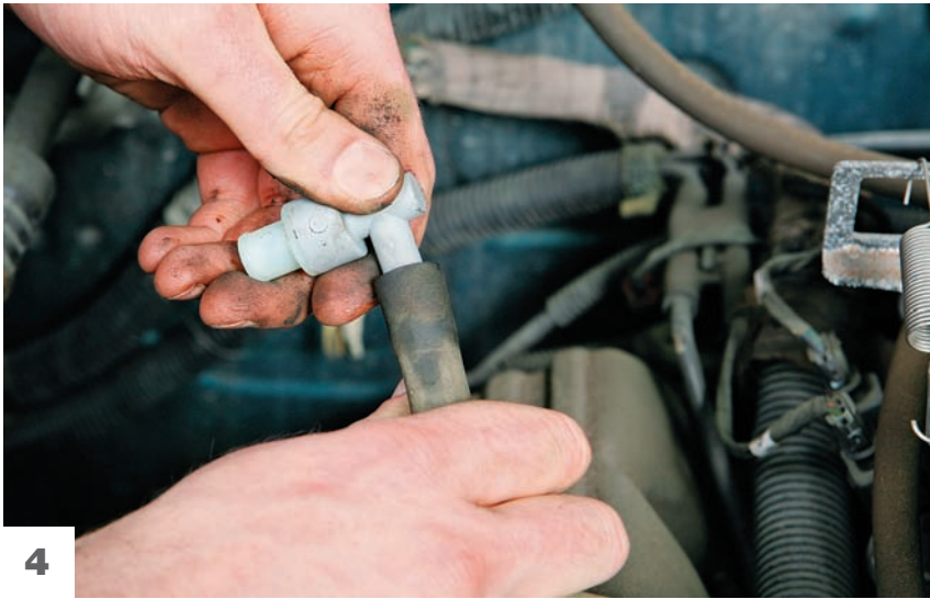
Push the new valve into the hose.
