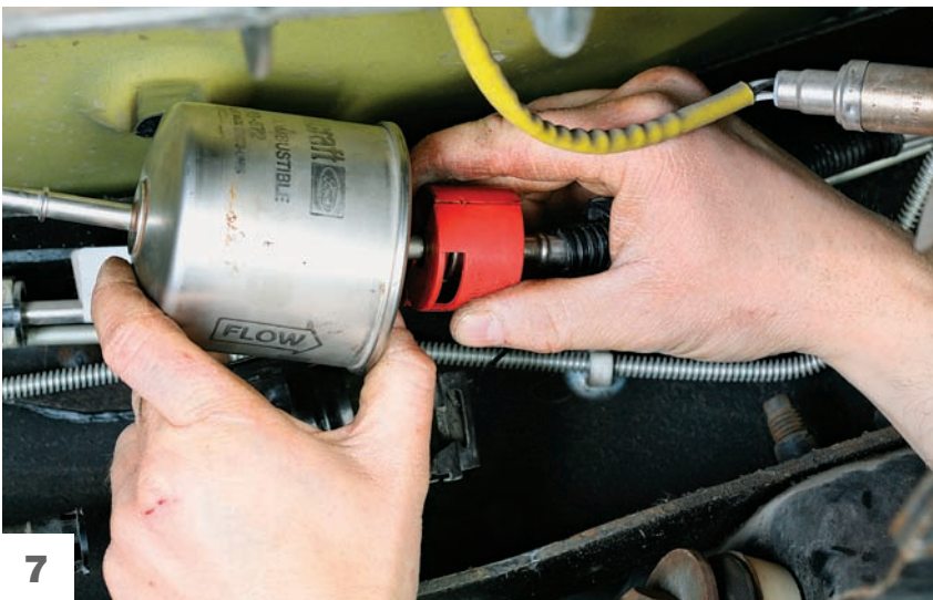
The front fitting uses a round spring clip that resides inside the fuel line where it connects to the filter. This type of fitting requires a special, inexpensive tool. Open the tool, fit it around the fuel line, and then press a collar inside the tool up into the fitting holding the spring clip. This releases the clip and allows you to pull the filter free. Note: Some fuel filters reside in inconvenient places and may require a lot more work, such as disconnecting and lowering the fuel tank. If you buy the filter and find you are in over your head, stop before you disconnect any fittings. Any garage can change the filter for you. Your manual will tell you the service interval for filter replacement. Typically, it's 15,000–30,000 miles. To install the new filter, reverse the removal procedure.
