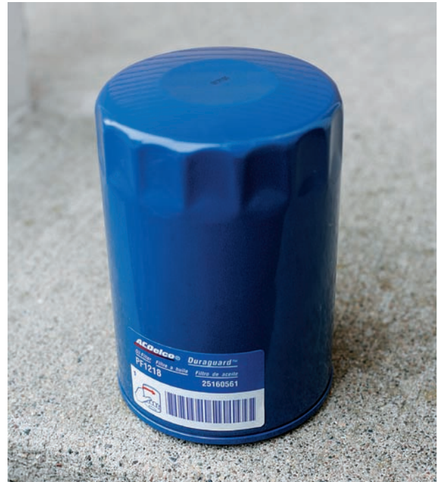
A typical automotive oil filter. Oil filters come in many shapes and sizes. Oil filter configuration depends on engine compartment space available as well as oil capacity as specified by the engine designer. In addition, oil filters may have check valves built into them to ensure that they stay primed during cold startup. Always make sure to use an OEM-comparable filter to ensure proper filtration.
