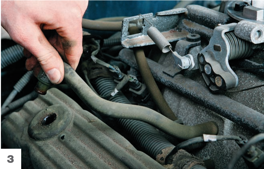
The valve may then be pulled from the hose running into the air cleaner.
