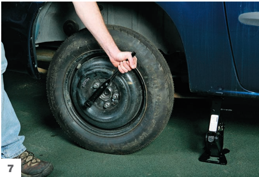
Lift the spare tire onto the wheel studs. If it's too heavy to lift by hand, sit on the ground in front of the wheel opening and use your feet to help lift the wheel into place. Thread all the lug nuts onto the studs and hand-tighten them with the lug wrench. Lower the jack until the tread makes contact with the ground, but don't set full vehicle weight on it. This way, the wheel won't spin when you fully tighten the lugs using a crisscross pattern. Double check that all the lugs are securely tightened, lower the vehicle, stow jack, throw the flat tire in the back. Tip: Fix your spare as soon as you can, even if it's not a "mini" spare. If you let it go, you may need a spare again and not have one.
