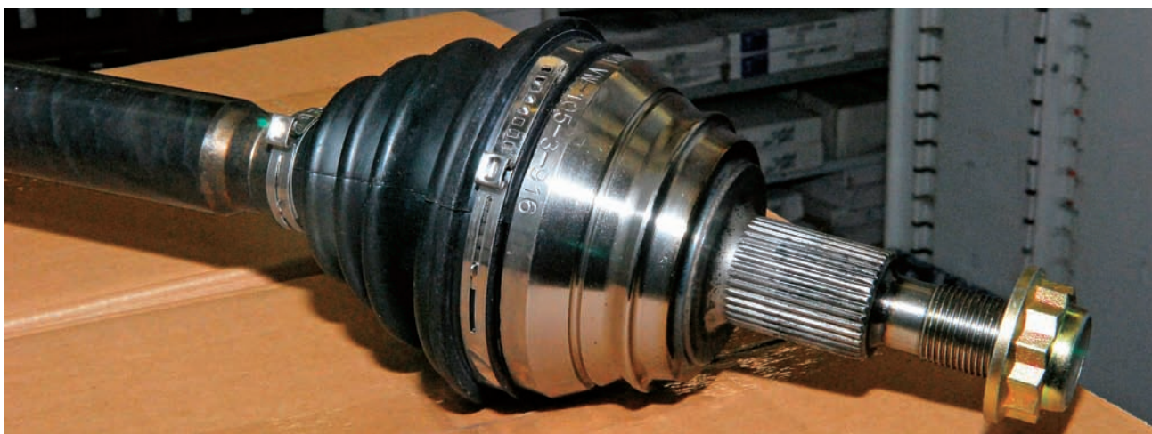
Rubber boots and bellows protect tight tolerance metal joints from weather elements, dirt, and road grime. If they tear or break from a projectile or just plain old age, the aforementioned elements are allowed to attack the joints and metal parts and wear them out in short order. Replace any compromised protective rubber boots immediately to avoid expensive part replacement.
