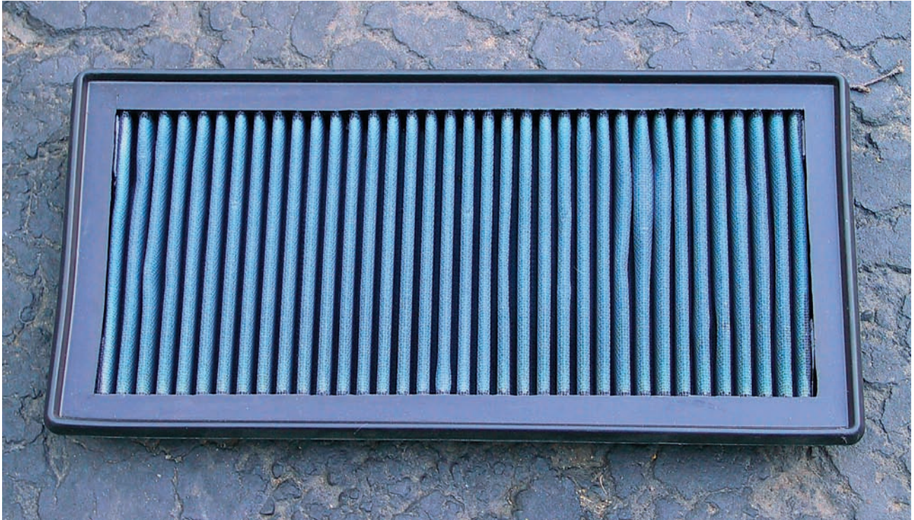
A typical automotive air filter: Because of fuel injection, never before has the air filter been so important to your car's performance and fuel economy. Computer-controlled electronic fuel injection measures airflow and engine operating environments to perfectly mix the air-fuel ratio to deliver maximum fuel economy, performance, and low tailpipe emissions. Replace the air filter according to the manufacturer's specs to realize maximum engine efficiency.
