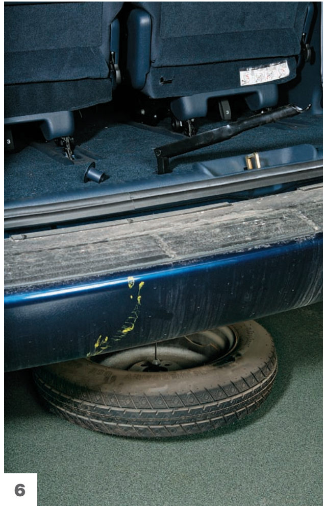
This lever releases the spare tire. Check your owner's manual for spare tire release procedures on your car.
