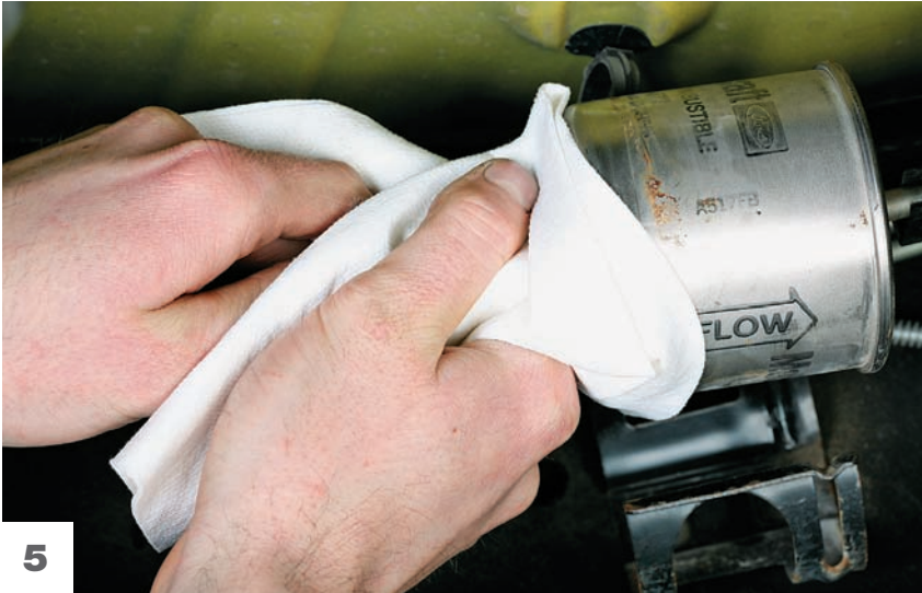
Place a towel over the fitting to avoid spraying gas and pull the fuel line off the filter.
