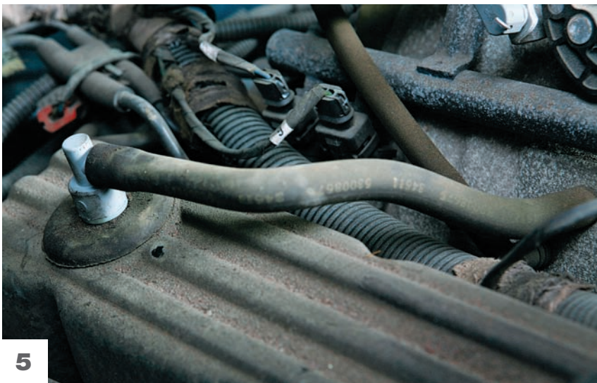
Press the other end of the valve into the rubber grommet in the valve cover. Make sure the valve is well sealed to the hose and valve cover.
