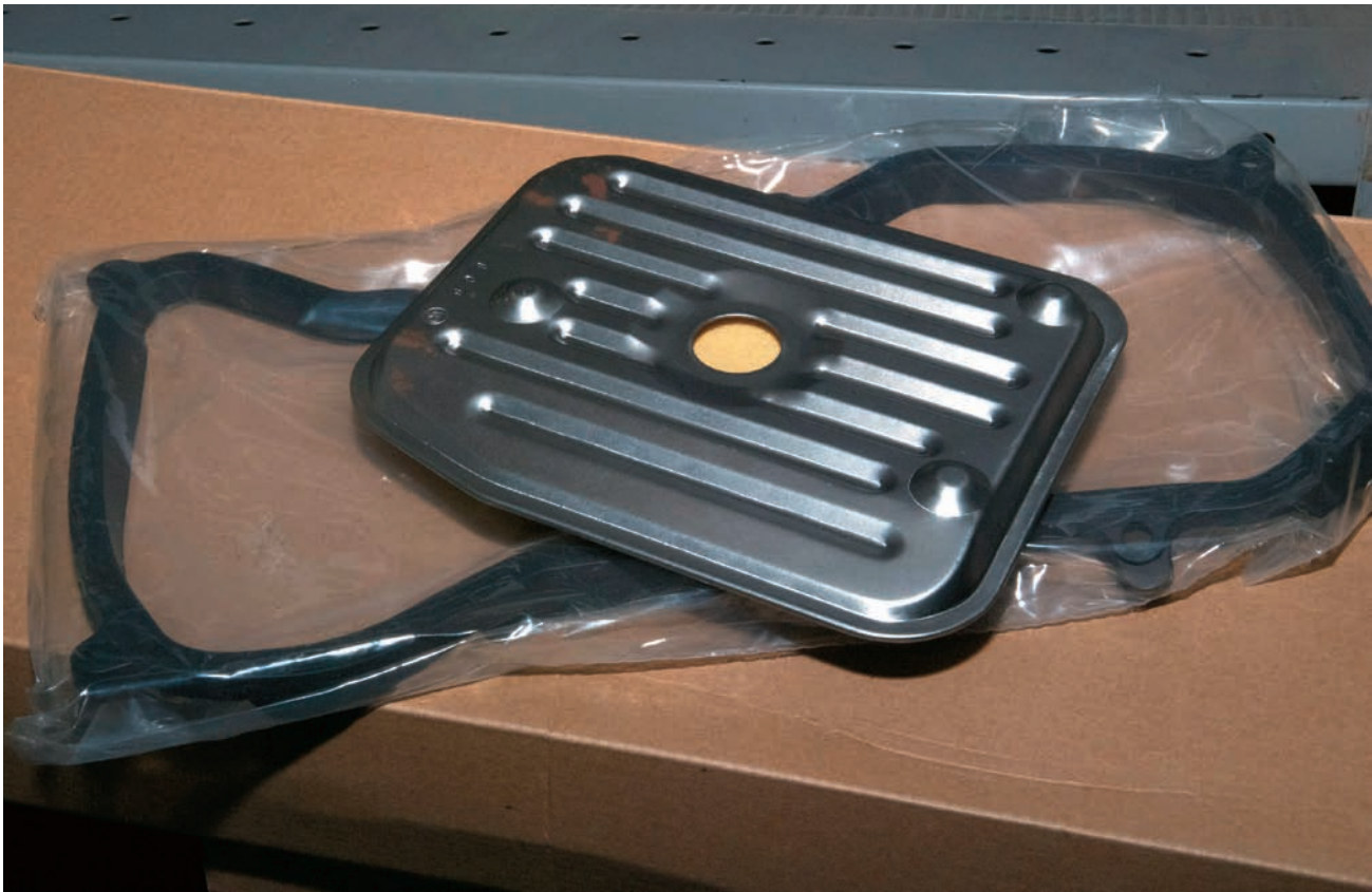
Transmission filters vary in shapes and sizes, depending on what model transmission they are designed to fit and filter. The filter is located in the transmission pan, where the transmission fluid is drawn into the filter to distribute throughout the unit after filtering it of impurities.
