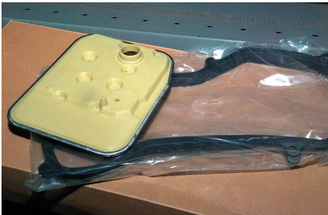
A typical transmission filter: Transmission fluid is nothing more than hydraulic oil designed to produce internal hydraulic pressure and cool and lubricate the unit. Transmissions by their very nature produce wear material that has to be filtered out of the fluid. This is the job of the transmission filter. Whenever a transmission service is done, use an OEM-quality filter to ensure maximum filtration. Transmission filters take various shapes to fit the pan configuration of a particular transmission.
