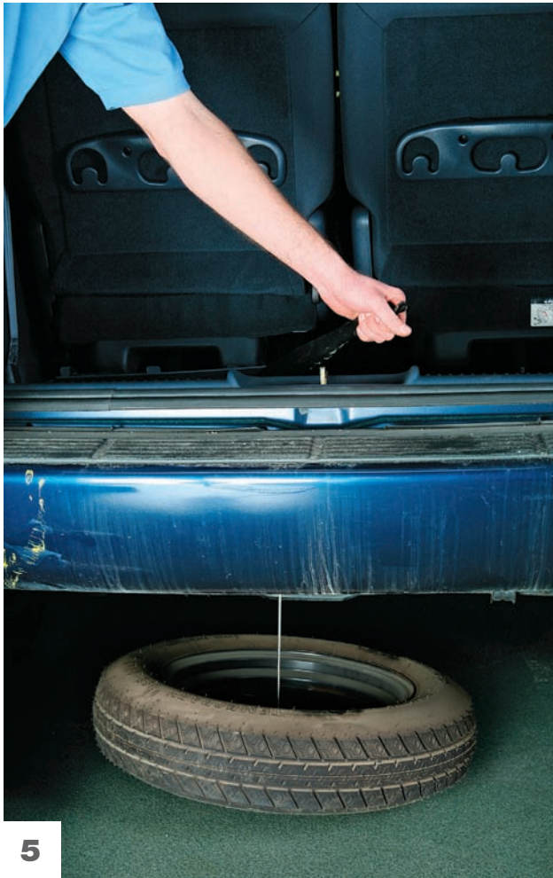
The spare tire in this Dodge Caravan is suspended underneath the van's rear end. To lower it, remove a plastic cap in the floor, exposing a nut that can be turned with the jack's wrench. Place the wrench on the nut and turn counterclockwise.
