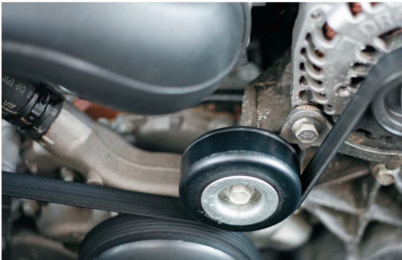
A typical serpentine belt with tensioner: The serpentine belt is a long belt that snakes its way through a series of pulleys, idlers, and a belt tensioner. This design eliminates the need for multiple drive belts. An effective cost-cutting design, serpentine belts tend to last much longer than traditional V-belts, usually upward of 50,000 miles.
