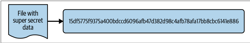
Figure 3-3. A file checksum; compare to Figure 3-2 , noting that the file contents have changed
