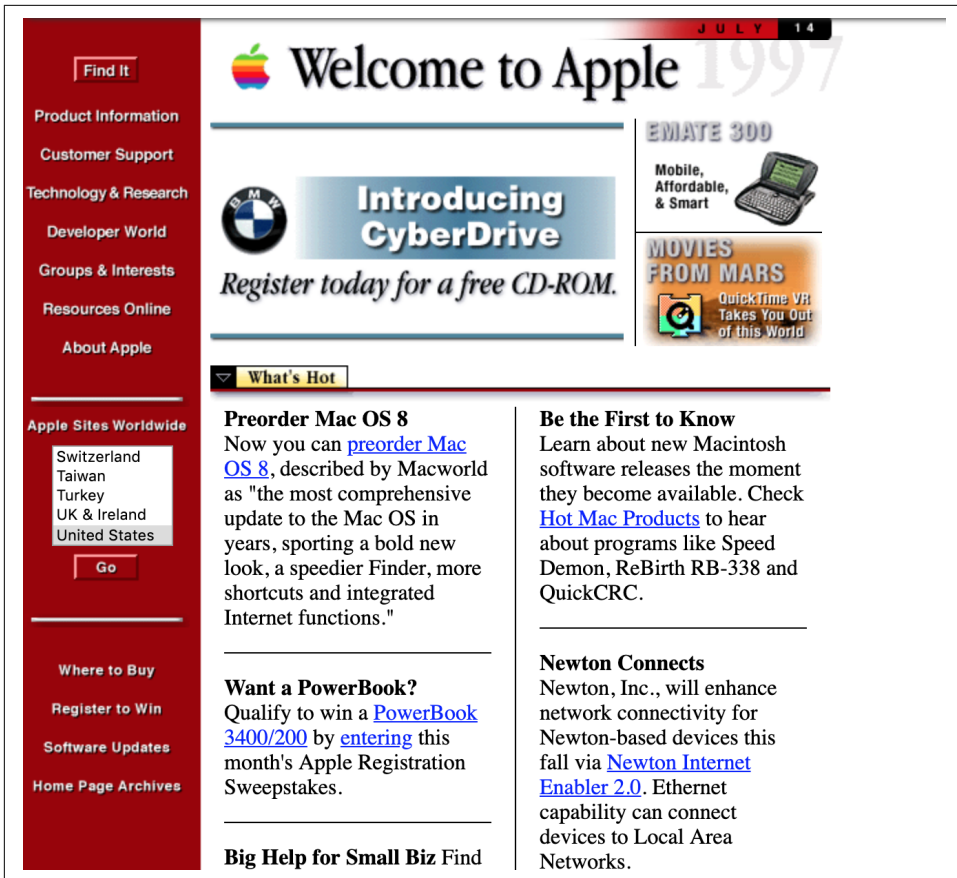
Figure 1-4. Apple.com website, July 1997; the data presented is purely informational and a user cannot sign up, sign in, comment, or persist any data from one session to another
